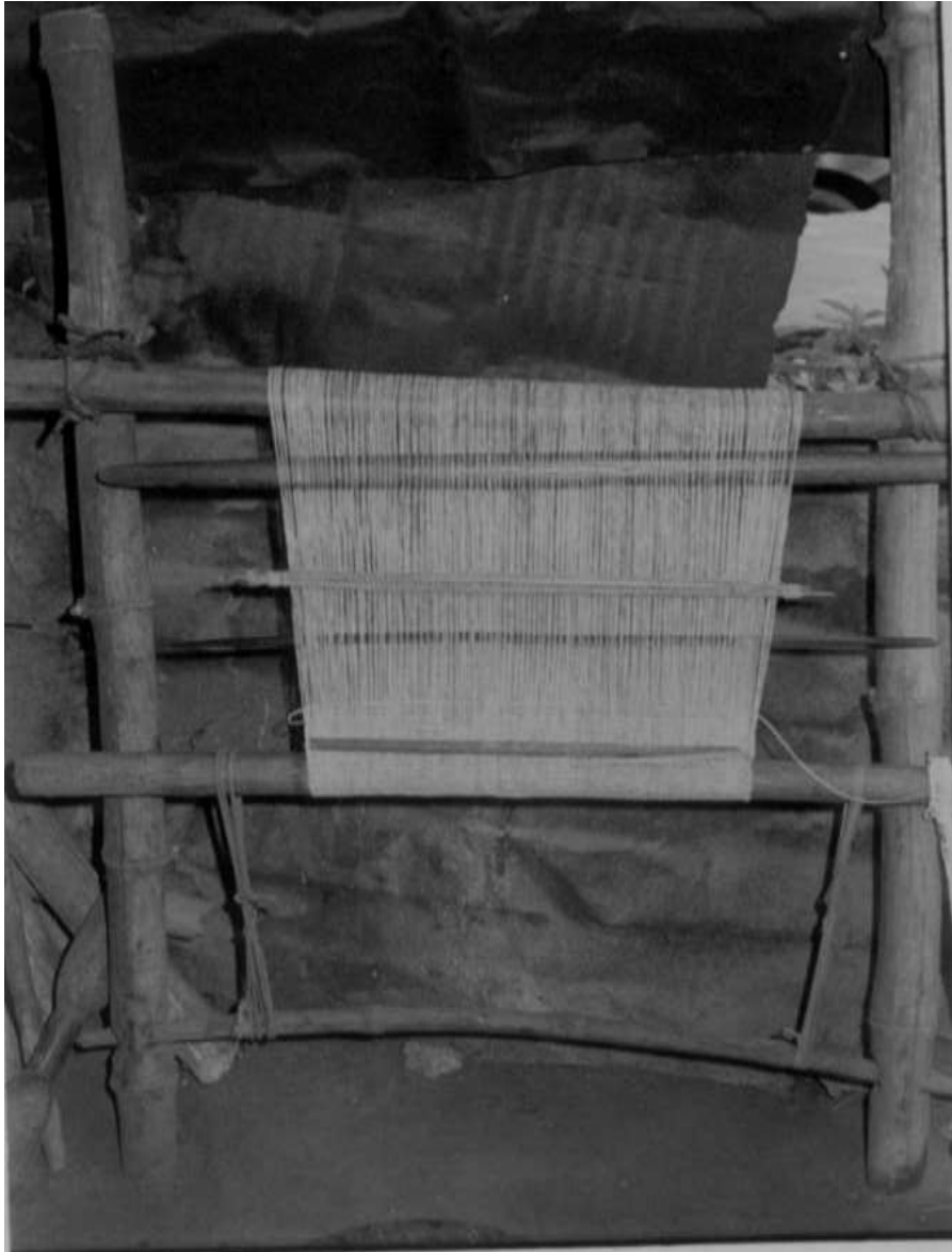
Fig 9a: Showing another different type of loom “Ogwere” the Aku weavers use. Here weaving has already commenced and the cloth being displaced on the loom “Ogwere”
