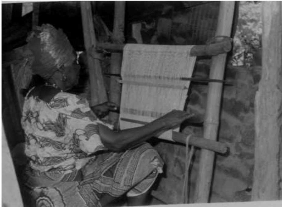
Fig. 14: Showing the Aku weaver in actual action of beating in every newly inserted wefts into the fell on the cloth. This process is repeated till the warp threads are use up and the weaving process is completed.
