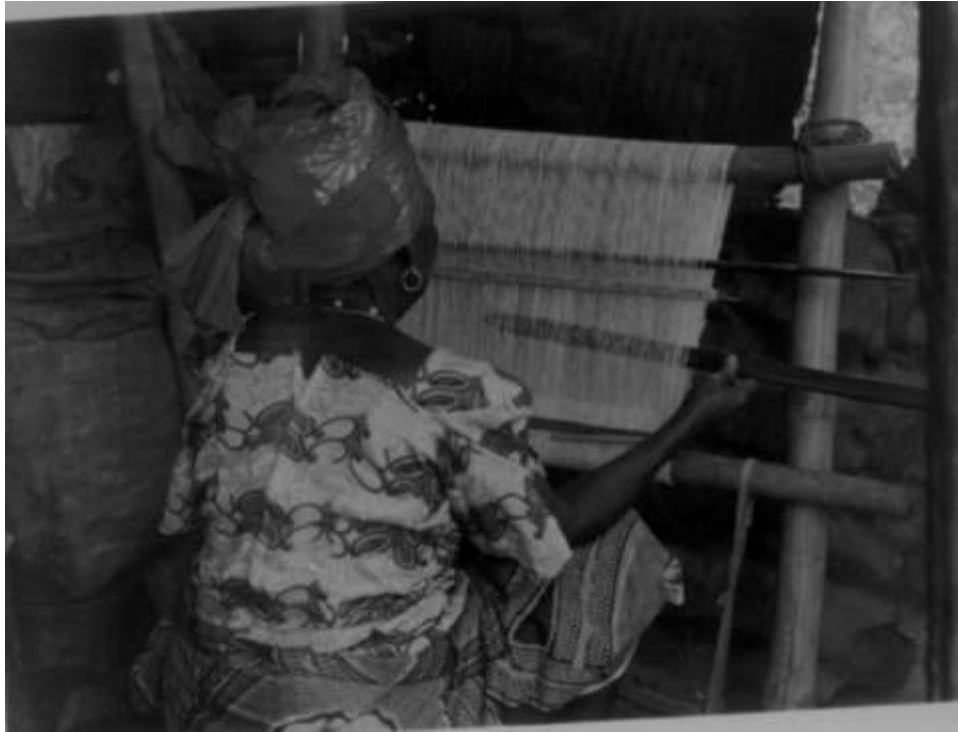
Fig 10: Showing an Aku weaver in action Madam, Enyivueku Igara of Igara Dimezie, Umu-Ehelete, Oshigo, Aku. Having completed the warping the primary heddle rod is woven in the manner described earlier, the number of heddle rods (shafts) required on a loom varies according to the intricacy of the patterning planned by the weaver.
