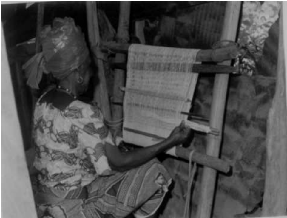
Fig. 12: Showing how the shuttle (Ukara) is being picking by the Aku weavers during the process of weaving in Aku. Here the shuttle locally called “Ukara” is being warp from right hand side and then to be picking from the left hand side through the shed.
