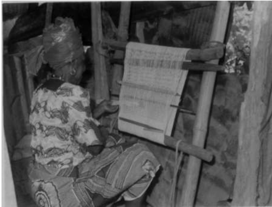
Fig. 13: Showing the Aku weaver operates on the principle of opposites. Here the shuttle "Ukara" is being warp from left hand side and then to be picking from the right hand side through the shed.
