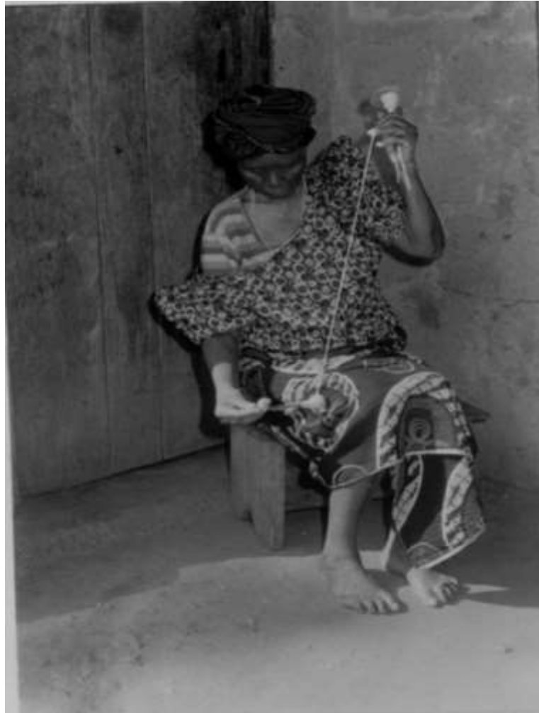
Fig. 4: Showing the Aku weaver spinning the thread into double threads which is the final spinning. The actual spinning is commenced by bringing the spindle into contact with the thigh and rubbing this spindle “Ntuturu” sharply against the thigh with the open palm of the hand. Three spindles “Ntuturu” are involved in this process, two spindles “Ntuturu” each with thread are raised up above the left hand while the remaining one is being held by the right hand and is into contact with the thigh and rubbing this spindle sharply against the thigh with the gripe palm of the hand with this, the actual spinning has commenced. This is locally known as “ifia-owu” in Aku.
