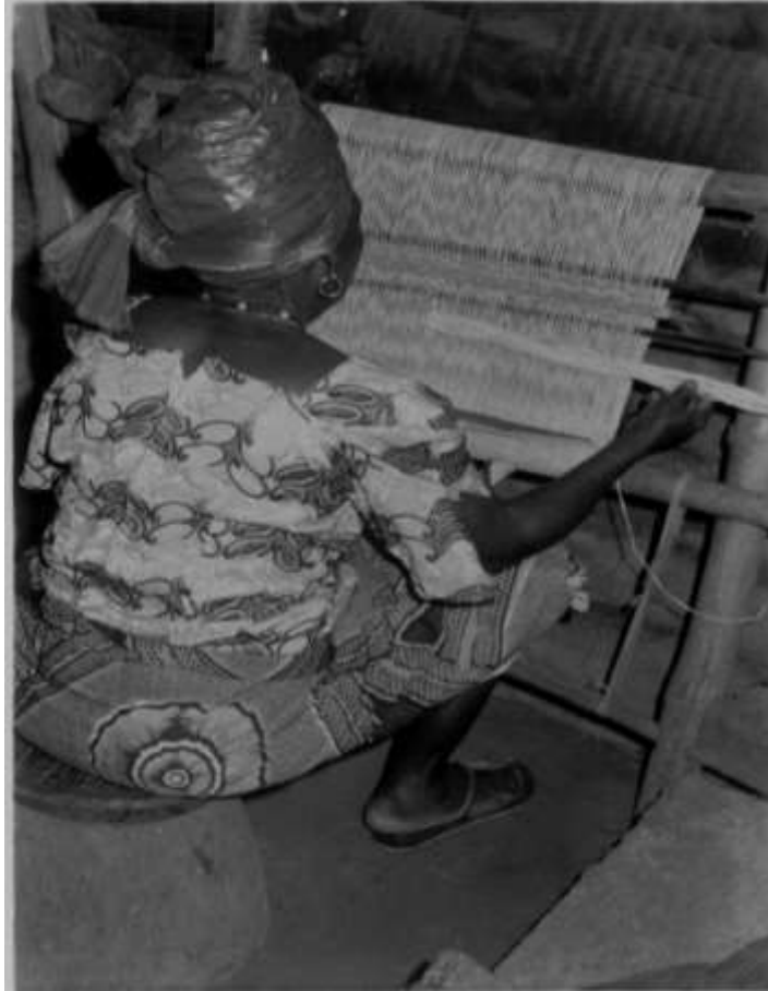
Fig. 11: Showing during the process of warping how the Aku weavers position the lease rods OR showing how the lease rods are being positioning by the Aku weavers during the process of warping.
